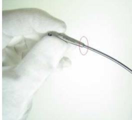
After sterilization the memory shaft turns back into original condition.
